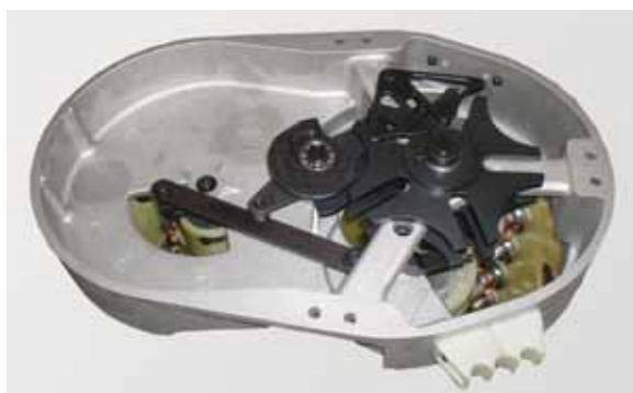
Fig 8. Geneva Wheel Mechanism
