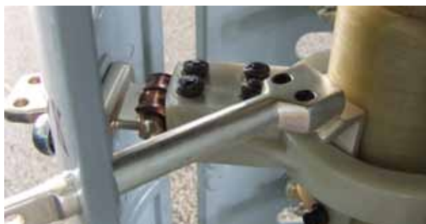
Fig 7 Tap Selector Contacts
